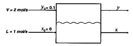
The molar gas and liquid flow rates, and the inlet mole fractions are given in the figure. Both the liquid and the gas phases are well mixed, and the equilibrium relation between y and x is given by  $y^* = x$ .
