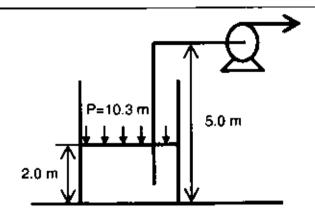
A storage vessel exposed to atmosphere (absolute pressure = 10.3 m of water) has a diameter of 3 m and is initially filled with water to a height of 2 m. The pump draws water from the vessel and is located at an elevation of 5 m above the bottom of the vessel. The frictional head loss in the suction pipe is 2 m of water. If the vapour pressure of the liquid at the temperature of operation is 3 m of water, then the available NPSH is
