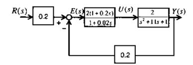
The steady state gain of the closed loop system, between output Y(s) and set point R(s), is
