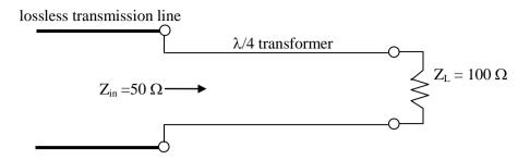
The characteristic impedance (in  $\Omega$ ) of the  $\lambda/4$  transformer is \_\_\_\_\_
