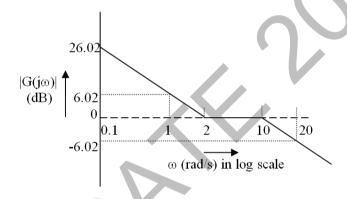
If the system is connected in a unity negative feedback configuration, the steady state error of the closed loop system, to a unit ramp input, is\_
