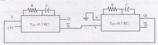
The frequency and the duty cycle of the signal at Q<sub>1</sub> will respectively be
