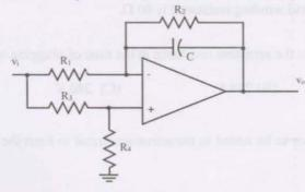
Q.80 If  $R_1 = R_2 = R_A$  and  $R_3 = R_4 = R_B$ , the circuit acts as a
