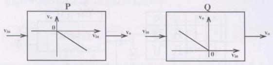
It is desired to make full wave rectifier using above two half-wave rectifiers. The resultant circuit will be
